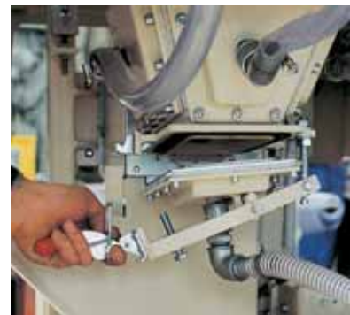
Maintenance door on the filling hopper
