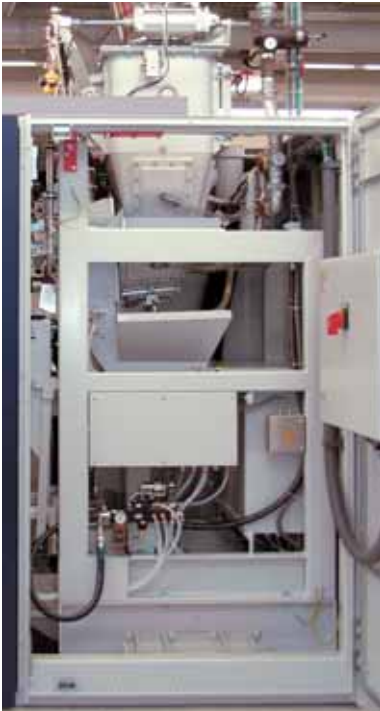
Air entrainment system
