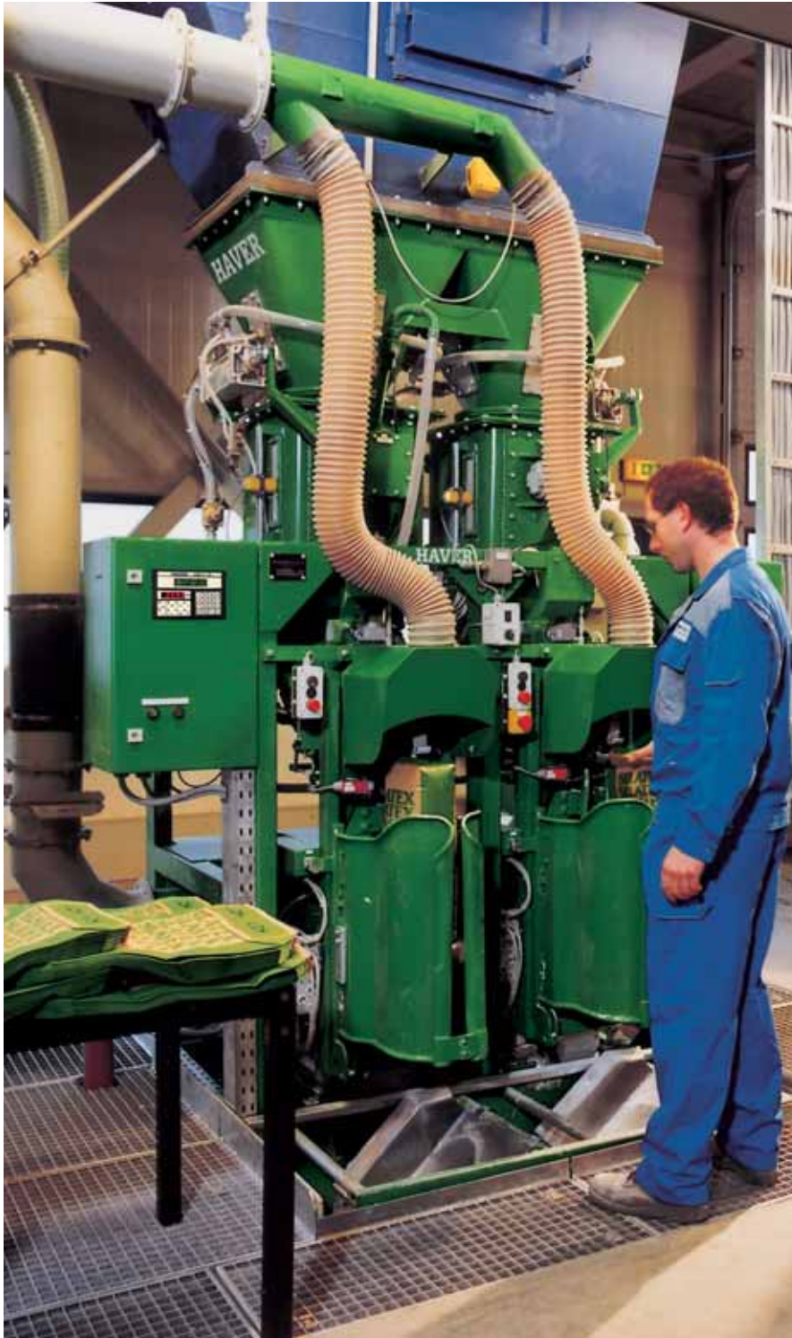
HAYER valve-bag filling machine using the air entrainment system outfitted with an automatic vertical bag discharger
