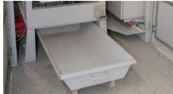
Spillage cart under the filling impeller
