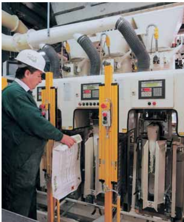
HAYER valve-bag filling machine with ultrasonic closing unit
