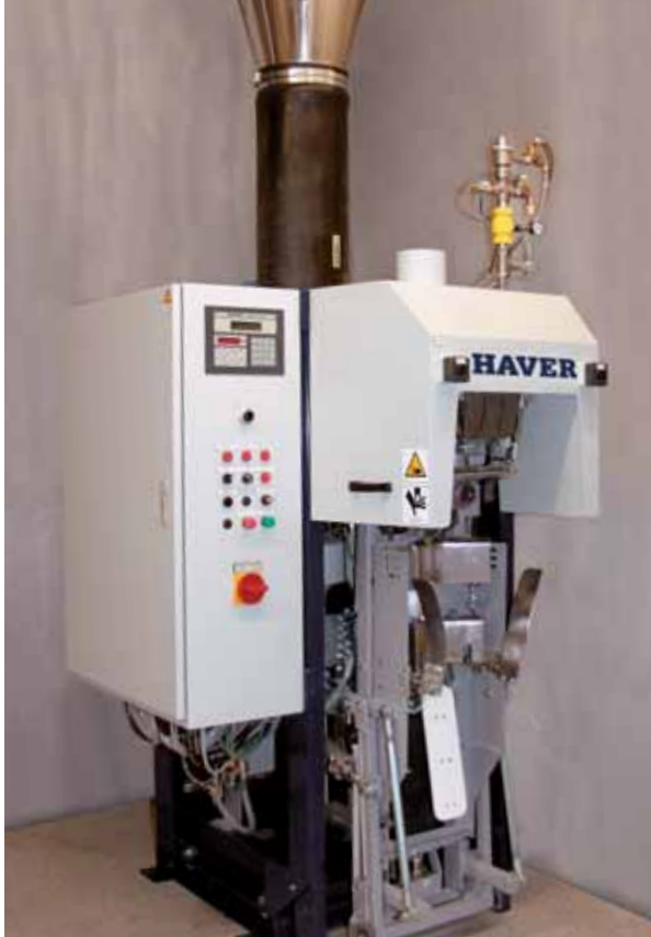
HAYER valve-bag filling machine with the horizontal impeller filling system
