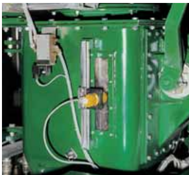
Pressure chamber with viewing window and fill level indicator
