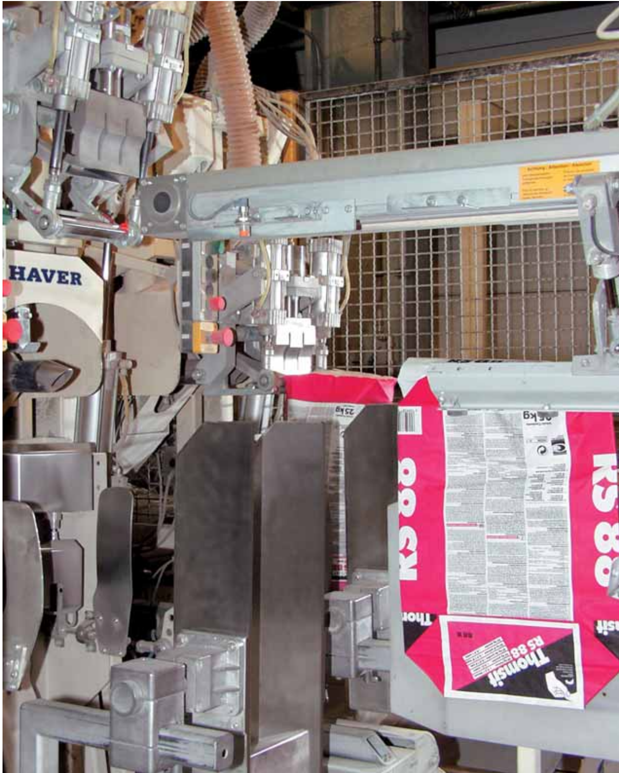
Fully automatic HAVER valve-bag filling machine with valve closing and automatic bag applicator
