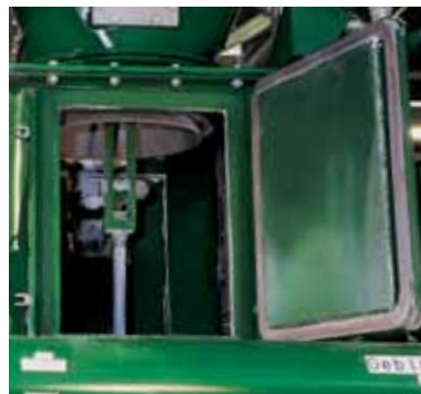
Pressure chamber with maintenance door
